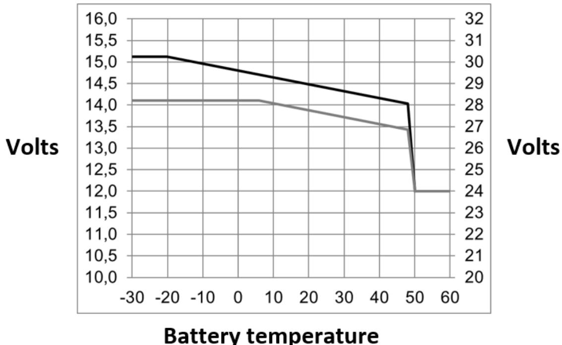
**EN:** Default output voltages for Float and Absorption are at 25 °C.
